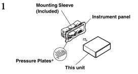
\* If the installed mounting sleeve is loose in the dashboard, the pressure plates may be bent slightly to remedy the problem.
